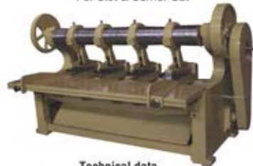
OHES Eccentric slotter For Slot & Corner Cut
