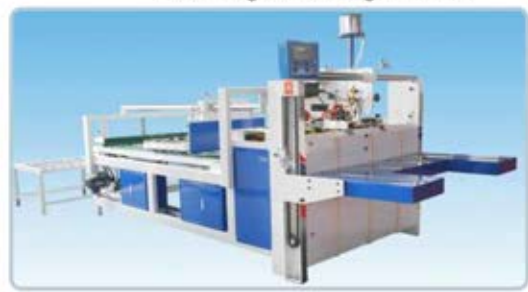
SAFGU Semi Auto Folder Gluer For Gluing and folding of Boxes
