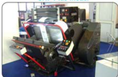
Machine with Fully Heated Stationary Platen for Plastic Cut / Crease
