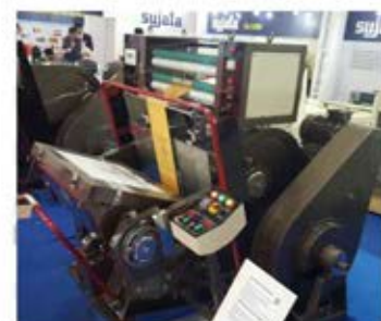
New stepper motor drive with Computerised Foil movement for fully use of Foil film and micro printing jobs.
